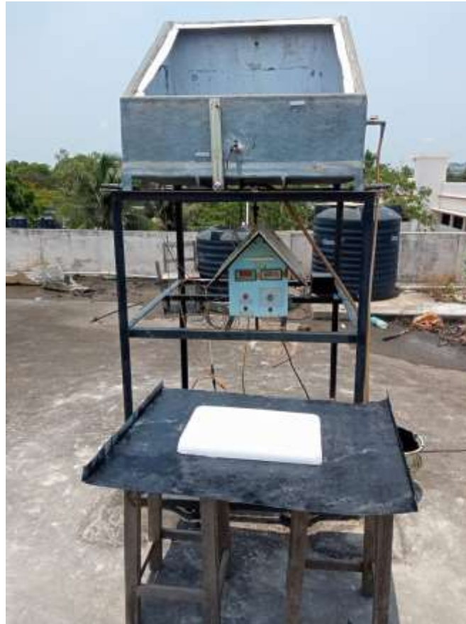
Fig 4.10 Photograph of solar still with wooden tetrahedrons
