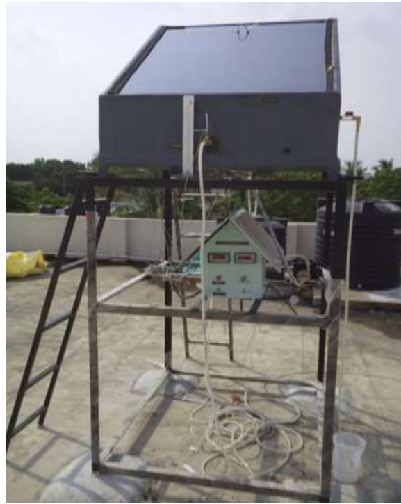
Figure 1b: Photograph of the working solar still.
